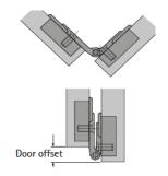
Fast assembly concealed hinge Intermat 9935 for door thicknesses up to 43 mm
